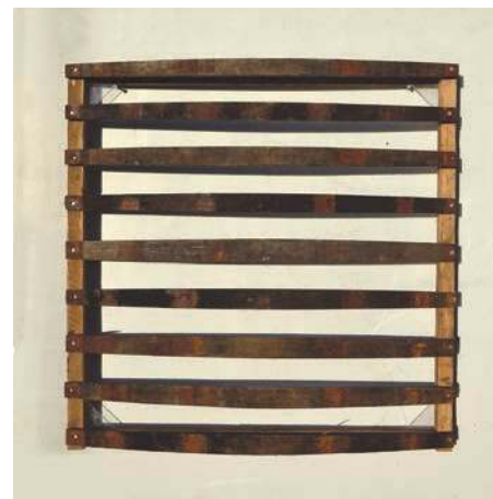
Narrow open (stave width: 25, spacing: 40)
